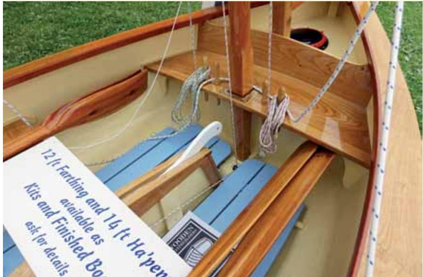
collar in the mast thwart acting as the fulcrum, thus moving the CE forward and allowing the boat to be perfectly balanced when una-rigged. As you can see from the silhouettes, the mast is freestanding with running rigging only, which facilitates this manoeuvre. (A move from a sprit boom set-up to the balance lug would probably be effected onshore, not afloat.)
