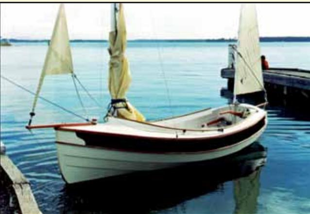
angles to rest the sore backs that so many of us suffer from, the seats are sealed to provide buoyancy, as is the raised deck area forward of midships that is large enough for the two of them to bed upon, and there is a huge locker under the foredeck where larger items can be stowed behind the hatch to keep them all dry.
