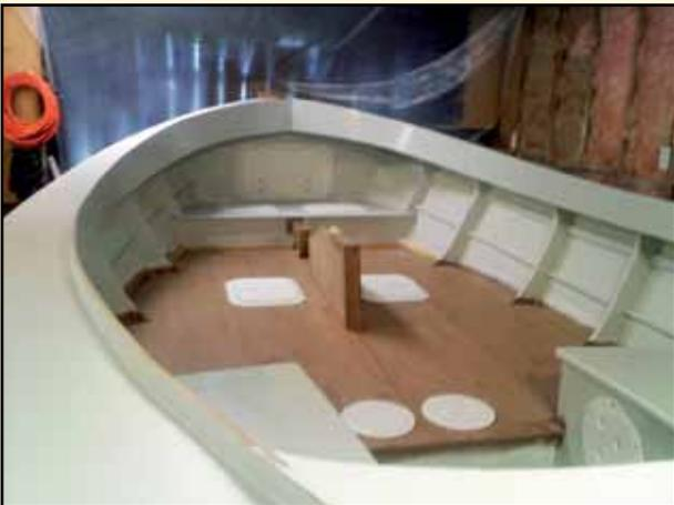
A view of the huge interior of Chip Matthews' PILGRIM, the buoyancy tanks under the seats and decks are sufficient to float the boat stable and upright even when fully swamped, an essential for an undecked boat that ventures into open waters. © Chip Matthews
