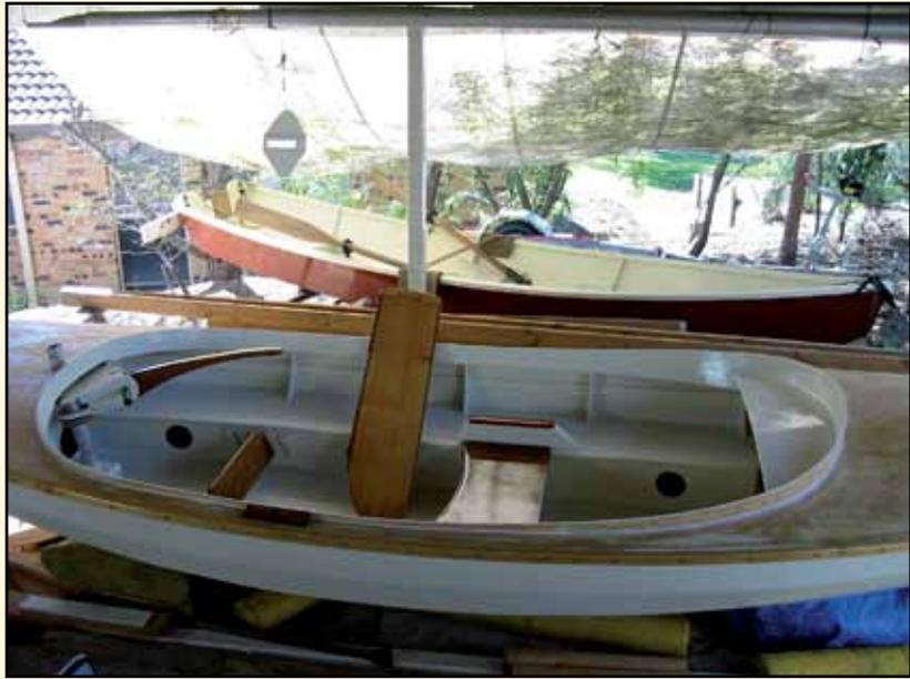
*With the removable rowing seat and foot stretcher lifted out and stowed, WALKABOUT has a very nice comfortable space in which to lie down. Note that builder Wayne Jorgensen found that his WALKABOUT was faster under oars than the JW-designed SEAGULL behind, and that boat's no slug either.*
