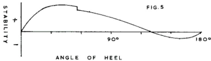
The negative stability beyond 120 deg. could be eliminated with a masthead float but this would complicate the design and seems hardly necessary bearing in mind that the chances of a capsize are small anyway.
