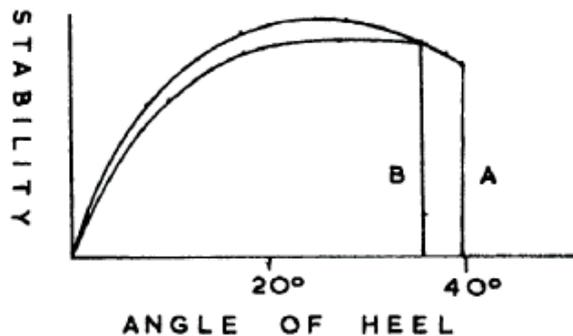
Figure 1 shows the stability curves of hulls A & B with the low freeboard which is
