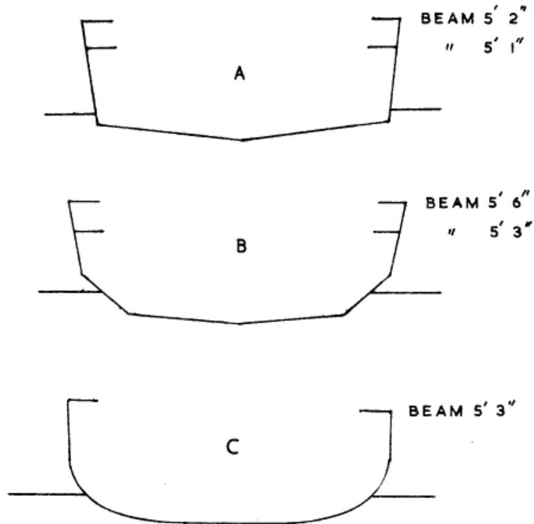
Three types of hull section are chosen for purposes of comparison, which I hope will be representative regarding their relative characteristics. It is assumed that 6" side decks are provided and that boats are laden with a full range of cruising gear. Hull C is that of the traditional clinker built dinghy.
