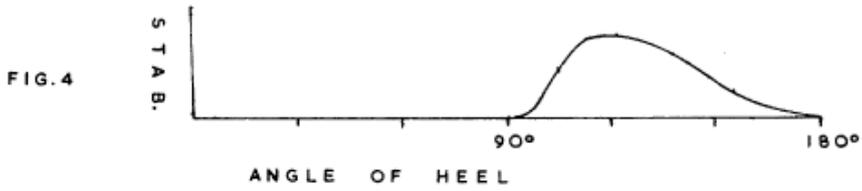
The mast has a section 2 3/4" x 2 1/4" and is 17' 6" long. If fully submerged and horizontal, it would have a buoyancy of 40 lbs. at about 10' above the C.G. of the boat, giving 400'lb righting moment, equivalent to the righting effect of a crew member sitting out. If the mast curve is now added in, the overall curve for the boat plus buoyancy is as figure 5.
