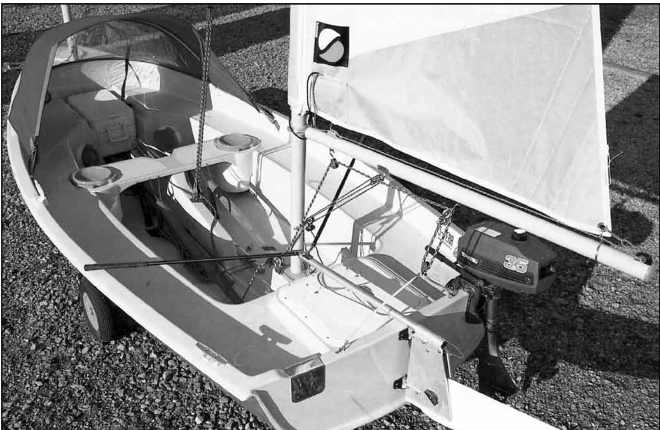
*The well-built, well-appointed CRUZ. A boat worth improving, especially now that it is no longer made and secondhand prices seem to have fallen as a result. Plenty of room for the secure fixing of ballast under the thwart.*
