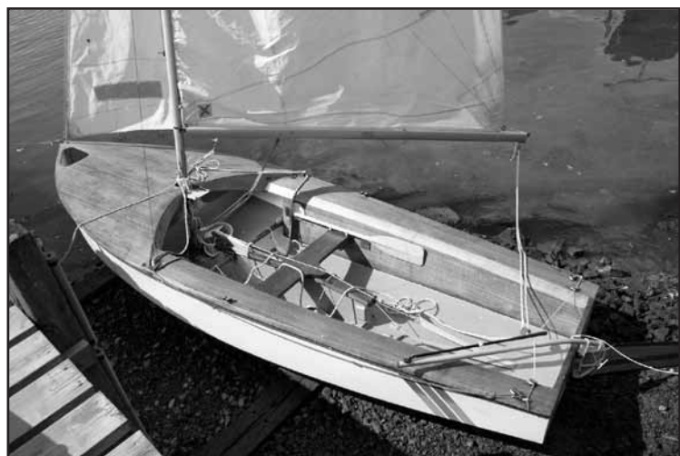
Cockpit layout for one of the last original SEAFLY hulls built.
