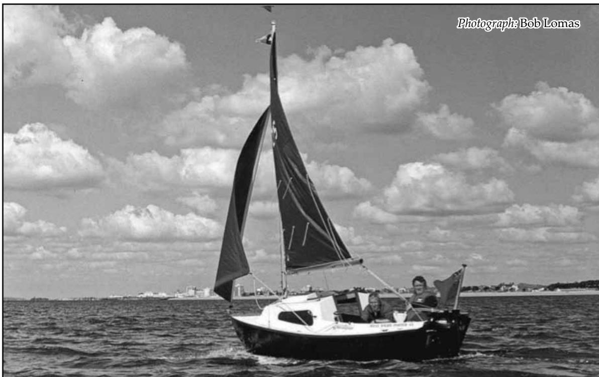
over 15 feet LOA, with a beam of 5 ft 6 in. Weight is around 650 lbs/296 kilos unladen.
